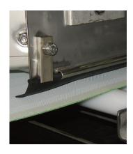
4 Side Seals - Replaceable rubber side seals prevent sludge from spilling off the sides of the moving drainage belt. A clamp is used to hold these seals in place for easy removal and installation.
