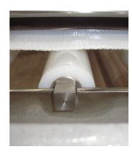
3 Belt Support/Wiper Bars - The dewatering belt is supported on abrasion-resistant, replaceable polyethylene wipers to enhance dewatering by constantly breaking the liquid surface tension. Wipers can be rotated providing multiple wear surfaces.
